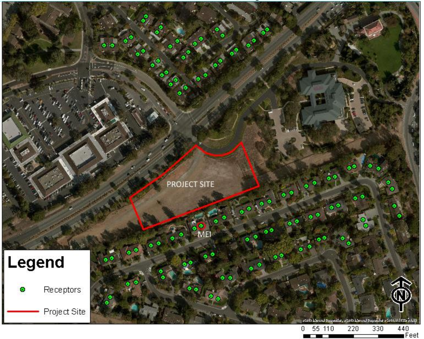
Figure 1. Project Construction Site and Locations of Off-Site Sensitive Receptors and Maximum TAC and PM 2.5 Impacts
